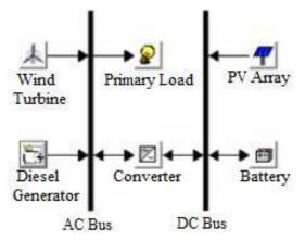
Figure 2. Single line Diagram of hybrid enegy system
